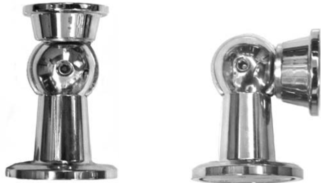
#34.MDHL in polished chrome Magnetic door holder Wall or floor or ceiling mounted; For medium weight doors distance: 75.5 mm - 3"high . Brass base material, except for magnet Cup in receiver part galvanized steel.
